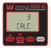
4. You should now see the CALC display. In order to set the unit to grains, press the MODE button until the display shows "3" as seen on the left. Press ENTER, then the ON/OFF button.
