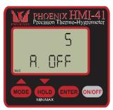
3. Press ENTER to display the A. OFF (automatic shut off) screen. You can adjust the number of minutes you want the unit to remain on if inactive. Then press ENTER.
